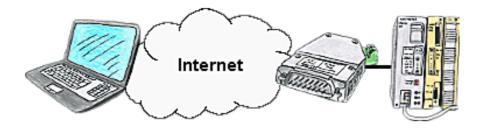
You have access to a on-site network and your PLC has no LAN-connection? No problem, plug the S5-LAN on the PLC and you will have immediate access to the PLC from afar.
